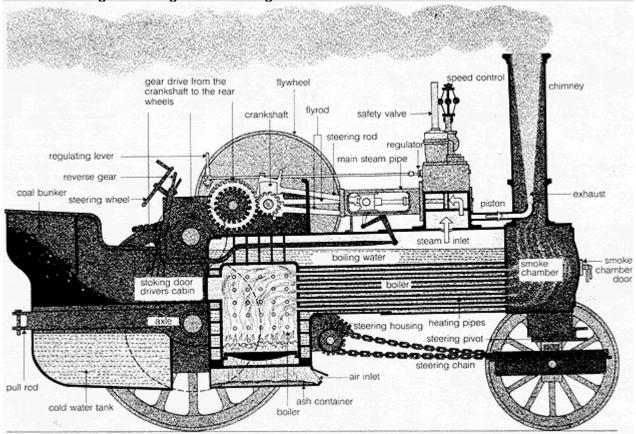
The driver of the steam engine or stoker shovels the coal through the stocking door into the boiler. The coal is being burnt.
