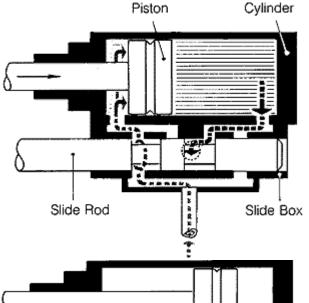
Just before the piston reaches the end of it  $\exists$  travel, on the extreme right, the slide valve cuts off the steam from the boiler. This is the point, where the crank is at the limit of its movement and is known as Top-dead-centre or Bottom-dead-centre? Referring to the two possible geometric positions. The flywheel carries the crank over this critical position by the energy it has stored from previous power strokes.
